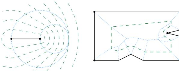
Figure 2: (Left) The variable-radius Voronoi diagram (blue, dotted) of a line segment and its two incident vertices. A family of offset curves is shown in green and dashed. (Right) The variable-radius Voronoi diagram inside a polygonal input with weighted vertices.
