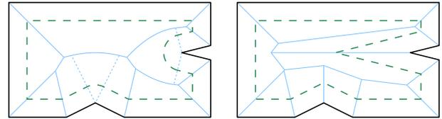
Figure 1: The Voronoi-diagram (left) and the straight skeleton (right) of a polygon enable efficient computation of constant-radius and mitered offsets (dashed).
