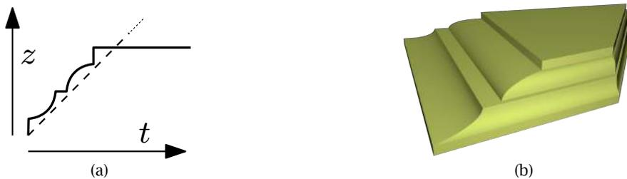
Fig. 4: (a) The height function used for obtaining the surfaces shown in Fig. 3(f) and 3(l). The standard height function which results in the roofs of Fig. 3(a) and 3(g) is shown by a dashed line. (b) Mitered chamfers based on a multiplicatively weighted straight skeleton also using the height function from (a).
