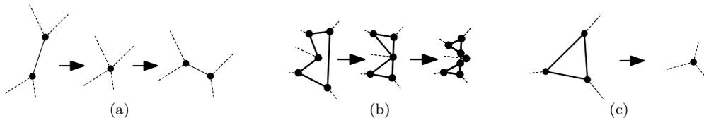
Fig. 2: Edge event ??, split event ??, and face event ?? during the wavefront propagation.
