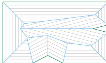
Fig. 1: The straight skeleton (blue) of an input polygon (green); several wavefronts are shown in gray.
