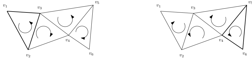
Figure 4: Two triangle strips: The left strip starts from the left and is (v_1, v_2, v_3, v_4, v_5, v_6) , the right strip starts from the right and is (v_6, v_5, v_4, v_3, v_2, v_1) .
